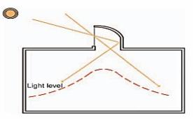
**Figure 7.** A single-sided roof monitor system designed to allow winter sunlight to enter but not summer sunlight.
