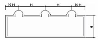
Figure 6. Rule of thumb for spacing skylights to obtain uniform light distribution beneath multiple skylights.
