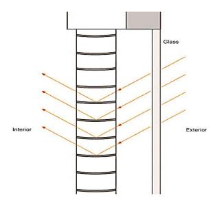
Figure 2. Light-redirecting louver system.
