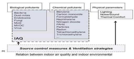
Figure 1. Source control measures and ventilation strategies; Model of causes of sick building syndrome; Relation between indoor air quality and indoor environmental
