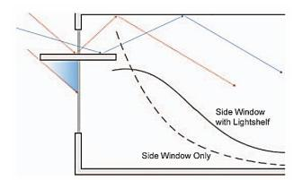
Figure 10. Daylight penetration from a combined lightshelf system.
