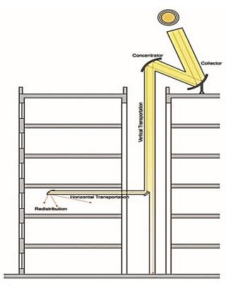
**Figure 5.** Alight pipe system with its various sunlight collection and light transport systems.
