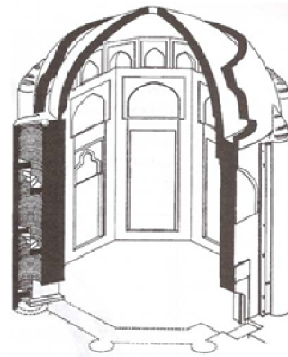
Figure 6: Using double-shell domes.
