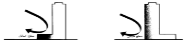
Figure 13. The highest and shortest points of the building on the windward front should be in the same direction so that the airflow reaches the street level.
